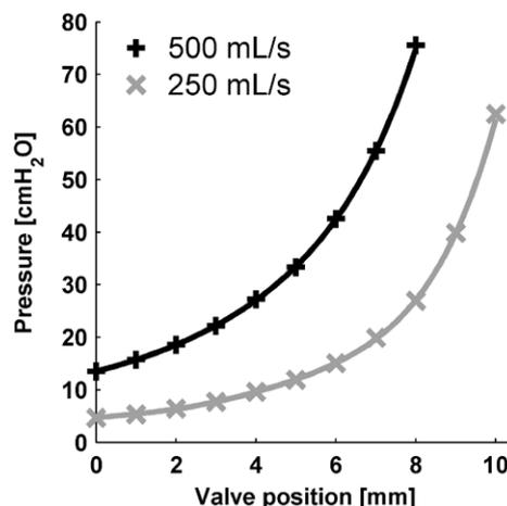
**Figure 1.** Flow- and position-dependent pressure drop across the FLEX system. The additional expiratory resistance of FLEX is determined by positioning of a cone inside an aperture. The resistance at a specific position equates the pressure drop divided by the respective flow rate. FLEX indicates flow-controlled expiration.
