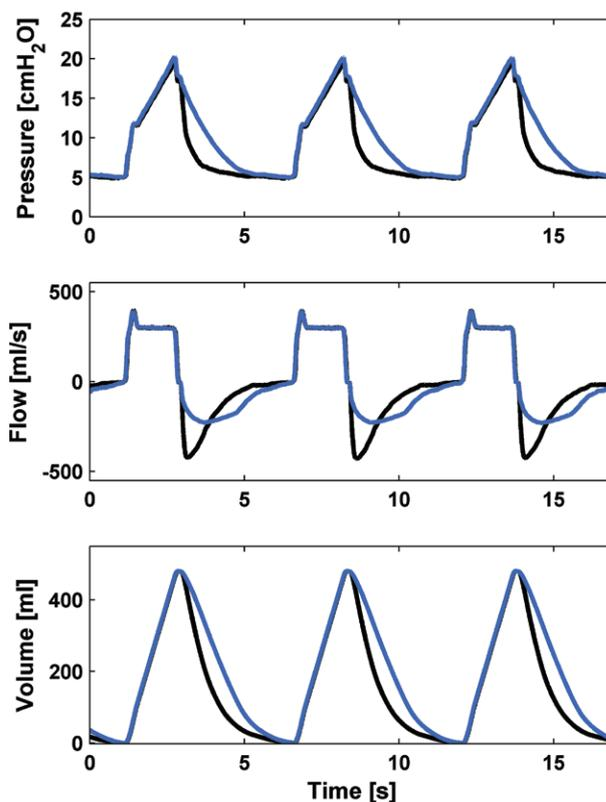
**Figure 2.** Airway pressure, flow, and volume curves of a representative patient ventilated with (blue) and without FLEX (black) at PEEP 5 cm H<sub>2</sub>O over 3 breaths. FLEX is characterized by a reduced expiratory peak flow and a linearized expiratory flow curve, a decelerated expiratory volume decrease, and airway pressure. FLEX indicates flow-controlled expiration; PEEP, positive end-expiratory pressure.
